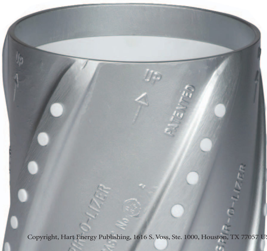
Figure 3. BladeRunner casing centralizers use Teflon-studded blades and liners to minimize sliding and rotational friction in ERD completions. (Image courtesy of Varel)
